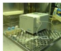
Microfluidic bioreactors connected to peristaltic pump and schematic of the general strategy
