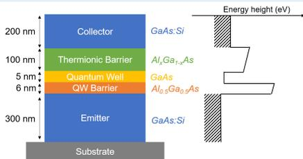
Fig.1. Layers of the thermionic device (left). Compared with induced energy height barriers (right). Heat is transferred from top to bottom.
