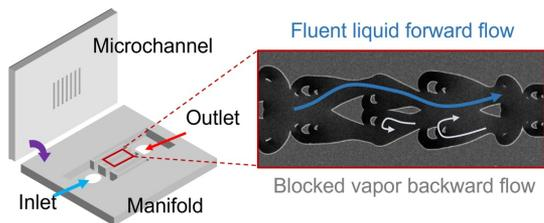
Fig.1. Channel with diode design
