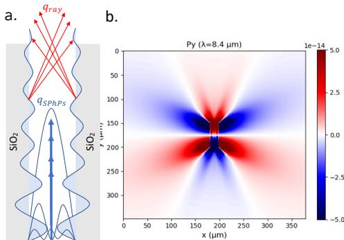
Fig.1.a. Scheme of a vacuum cavity between two identical polar materials supporting the in-plane propagation of SPhPs via cavity modes (blue lines). Classical and Planck radiation (red arrows) adds up to this latter contribution. b. Poynting vector mapping of the cavity effect for  $\text{SiO}_2$  at  $8.4 \mu\text{m}$ , maximal wavelength of SPhPs propagation. The cavity effect is isolated by dividing the impact of two independent walls.
