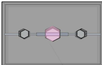
Fig.1. Porous scaffold embedded in collagen matrix in PDMS chip
