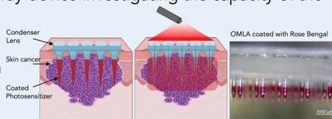
Fig.1. Schematic representation of PDT using OMLA (left) image of Rose Bengal coated OMLA (right)
