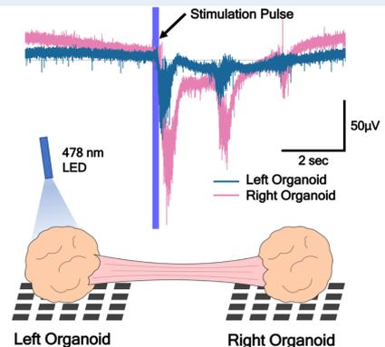
Fig.2. Optogenetic stimulation of the left organoid induces a burst that propagates to the connected organoid.
