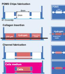
Fig.1. Microfluidics chips fabrication
