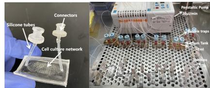
Fig 1: Biochip and perfusion set up
