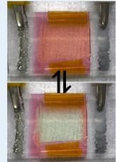
Fig.2. ECD architecture and pictures of color switching in a polyRu-based ECD
