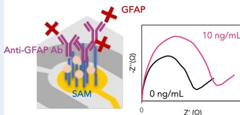
Fig.1. Sensor scheme (left) and change in EIS in the presence of GFAP (right)
