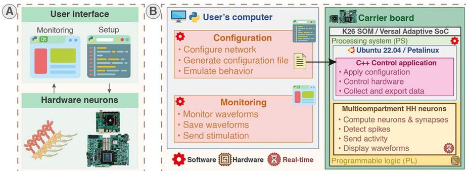
Fig. 1. System overview of the real-time hardware-based emulator for multicompartment Hodgkin-Huxley neurons.
