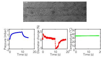
Figure 2: Image acquisition performed simultaneously with pressure, diameter, and temperature measurements.
