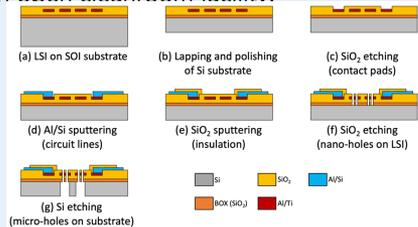
*Process workflow for fabrication of a coulter counter: lapping/polishing, top side holes etching, deposition, back side holes etching*
