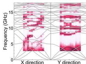
a. Optimization process of the phononic crystal based on inverse design method. b. Fabricated structure with optimized design c. Comparison between the designed phonon dispersion relation (gray lines) and Brillouin light scattering measurements (red color).
