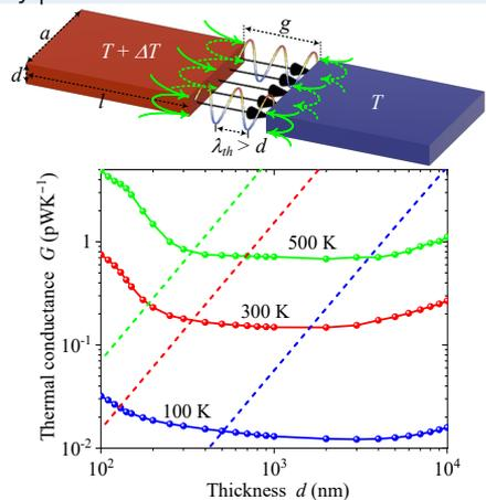
Fig. 1: (a) Scheme of two membranes exchanging thermal radiation through photons (wavy lines) and polaritons (green lines). (b) Thermal conductance as a function of the membranes' thickness.
