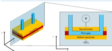
Fig.1. Schematics of the micro gap device.
