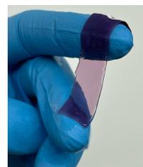
Fig.2. Ultra conformable semiconducting hydrogel
