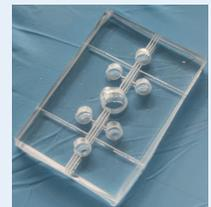
Fig. 1 – Microfluidic device
