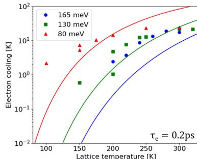
Fig.2. Experimental data (points) compared to curve of electron cooling in quantum well for different barrier heights.
