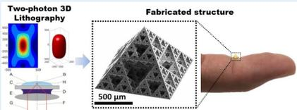
Microrobotic biosample handling by 3D printed polymer micro fractal pipette [1,2]
