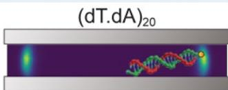
Schematic representation of the system under study. A tethered ds-DNA nanoconfined between two electrodes. The heat map represents the position of the redox marker.
