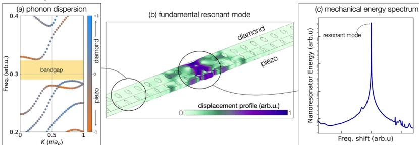
Quantum telecommunication interface formed by a double hybrid nanoresonator of diamond embedding color defects and a piezoelectric material (AlN). By exciting mechanical modes in diamond, the system behaves as a spin qubit.
