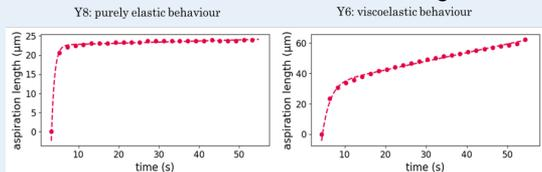
Micropipette aspiration experiment on different DNA hydrogel designs
