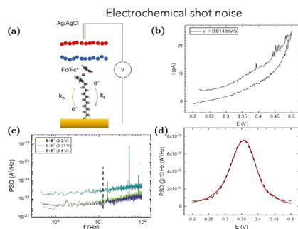
(a) FcC<sub>11</sub>SH SAM on gold. (b) CV of a FcC<sub>11</sub>SH SAM on gold. (c) Noise spectra measured at 0.014 mV/s (d) Noise versus potential at 10 Hz.
