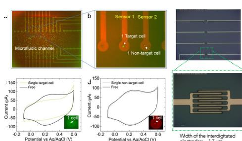
Figure 2. CV results to show the selectivity of the device.
