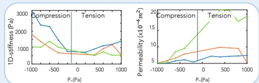
Fig.2 Physical properties extracted from different cellular hydrogels using a pressure measurement assay combined with a mathematical model [2]. These graphs show a clear asymmetry in the response of the hydrogels between compressive stress (negative pressure) and tensile stress (positive pressure).
