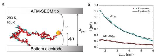
**a** Schematic representation of the experimental setup. **b** Experimental result of current as a function of the gap for ssDNA and dsDNA.
