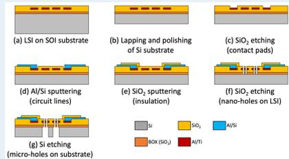
Post-processing workflow for fabrication of a couler counter: lapping, polishing, top side etching, deposition, back side etching
