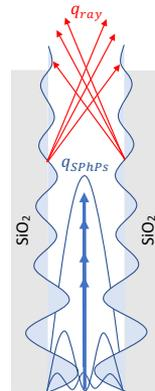
Figure 1 - Vacuum cavity between two polar materials supporting the in-plane propagation of SPhPs via guided modes (blue lines) and Planck radiation (red arrows).
