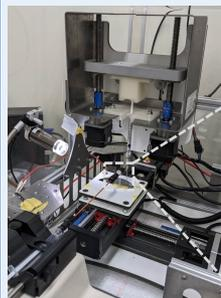
Predefined structures were obtained through additive manufacturing of DNA hydrogels.
