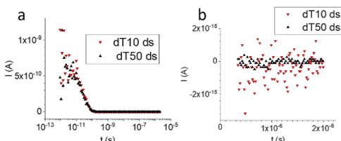
These two double-stranded (T sequences) have different lengths. They carry the same electrochemical marker. Though they show similar currents during a chronoamperometric measurement (a), they exhibit different noise signature (b).
