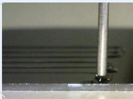
Figure 2: Experimental setup to print a DNA hydrogel with a predefined structure
