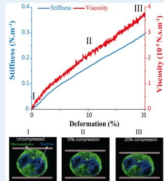
Fig.2: Mechanical characterization during intracellular visualization.
