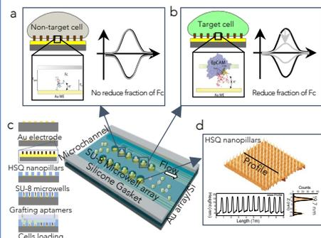
Figure 1. Principle of the single-cell EC aptasensor array.
