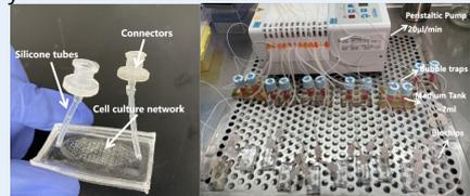
Fig 1: Photo of biochip and perfusion setup
