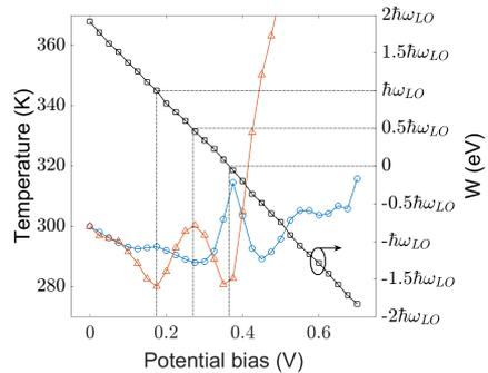
Fig. 2: Electron temperatures in the quantum wells as a function of bias. Energy difference  $W$  between the quantum wells ground state (black line).
