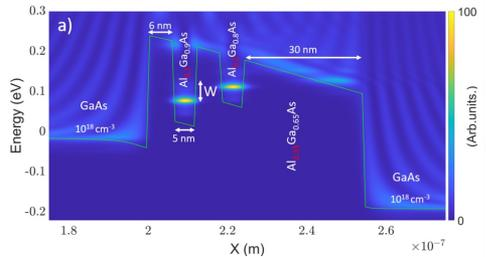
Fig. 1: Electronic density of states of the Quantum Cascade Cooler under a bias of 0.2 V.
