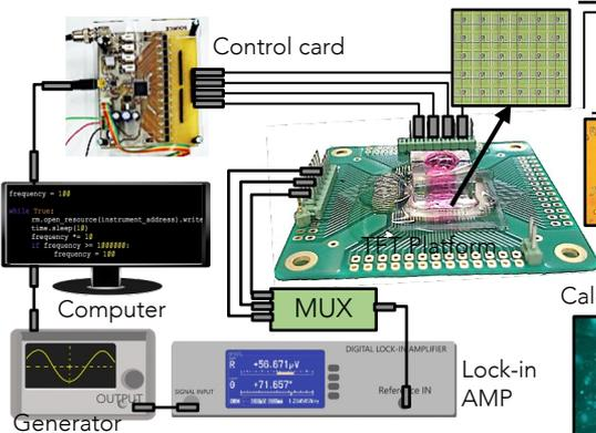
Automatisation of 2D bioimpedance measurements
