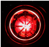
Top view of the inside of the VPS during the measurement at 1200 K
